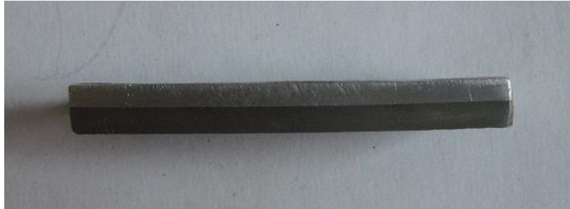
Fig.3: Aluminium-Steel bimetal plate, sample
